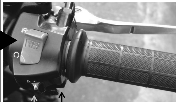
Remove fixing screws for existing throttle housing (usually located underneath)
