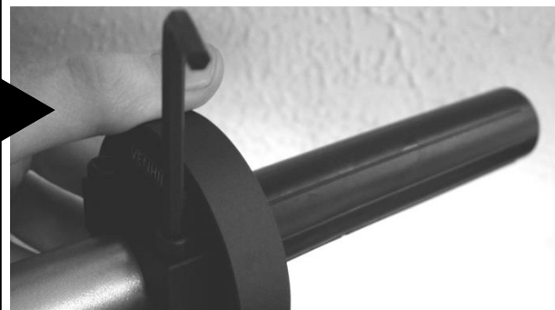
Loosen the 4mm Allen key clamp bolts, fit 888 to handlebar
